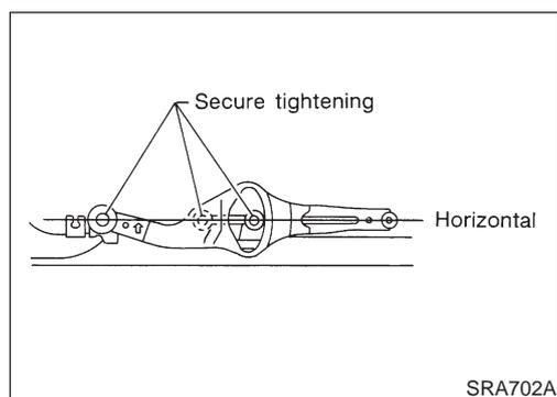
3. Place lateral link and control rod horizontally against torsion beam, and tighten to the specified torque.
