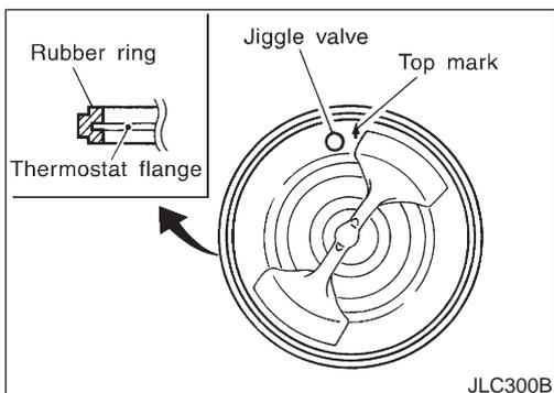
5. Install thermostat with jiggle valve facing upward.
