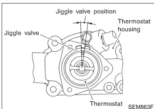
4. Install thermostat with jiggle valve or air bleeder at upper side.
