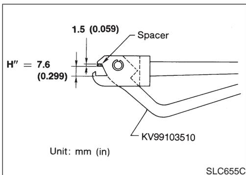
1. Attach the spacer to the tip of the radiator plate pliers A. Spacer specification: 1.5 mm (0.059 in) thick x 18 mm (0.71 in) wide x 8.5 mm (0.335 in) long.
