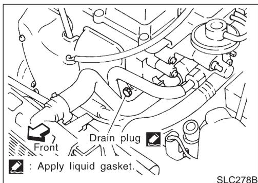
2. Open radiator drain cock at the bottom of radiator or remove lower radiator hose, and remove radiator filler cap to drain coolant.
