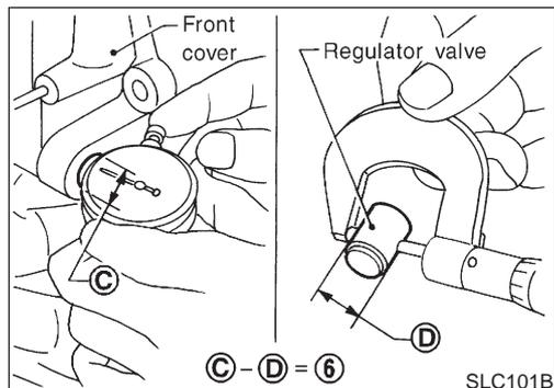
4. Check regulator valve to front cover clearance.
